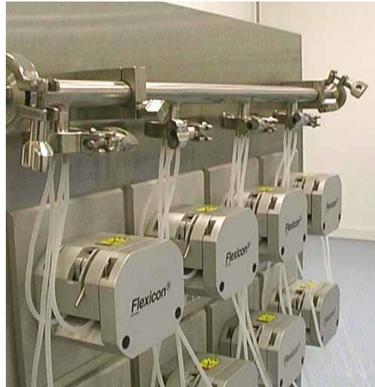
Trolley solutions are supplied for integration into new or existing filling lines fitted with up to sixteen peristaltic fillers
