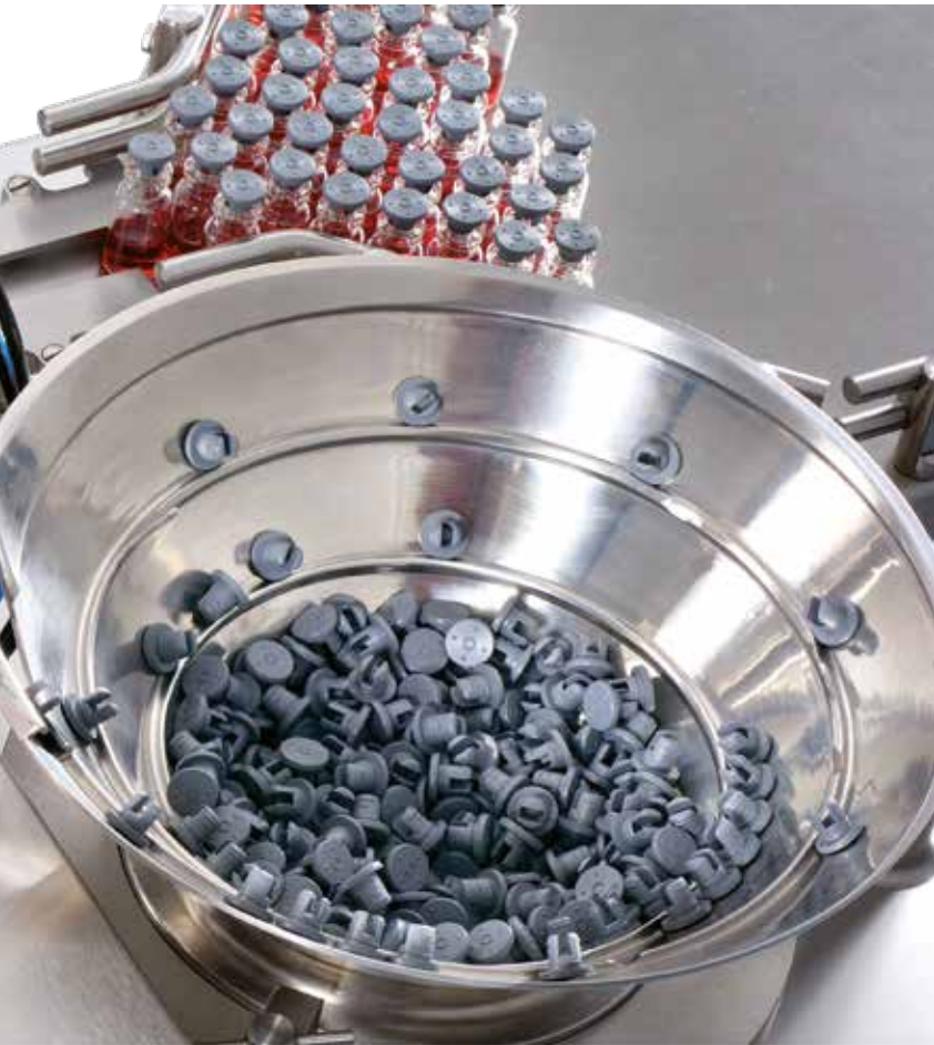
Stoppering with 13 mm and 20 mm stoppers requires no additional format parts
